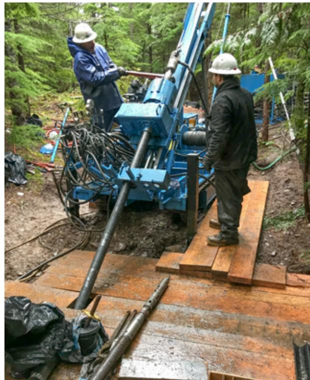
**Figure 7:** A small, hydraulic, track-mounted core-drilling rig was used in November 2018 to test the continuity and variation at depth of the nephrite bodies at the DJ project. Photo by J.-P. Jutras.
