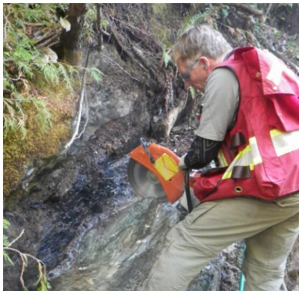
**Figure 8:** A portable diamond saw is used to extract masses of nephrite, shown here during initial sampling in October 2017. Photo by J.-P. Jutras.
