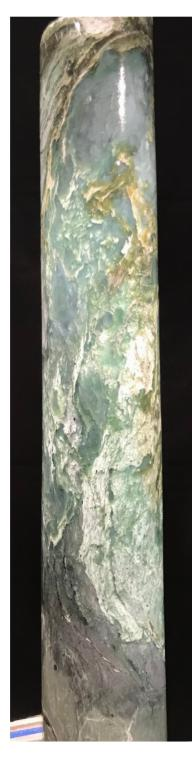
Drill hole L2DD2, polished core from 12.3 to 12.7 meters. Core diameter is 6.3 cm (HQ core).
