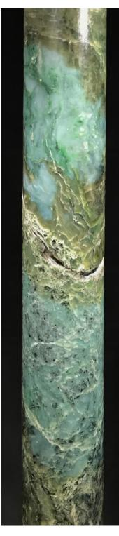
Drill hole L2DD1, polished core from 10 to 10.5 meters. Core diameter is 6.3 cm (HQ core).
