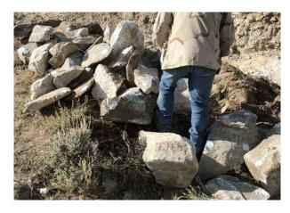
Jade samples from trench T1C bedrock laid out on side of trench for first pass review. All samples were marked in the field with a white marker to identify origin.
